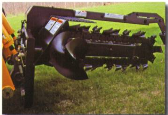
A new option for the XR-Series is a fixed mount design. This reduces cost, offers reduced weight, promotes even better stability, and is a more compact package.
